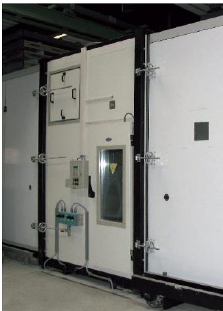
Figure A.1 Three-chamber climate simulator “hot box”
