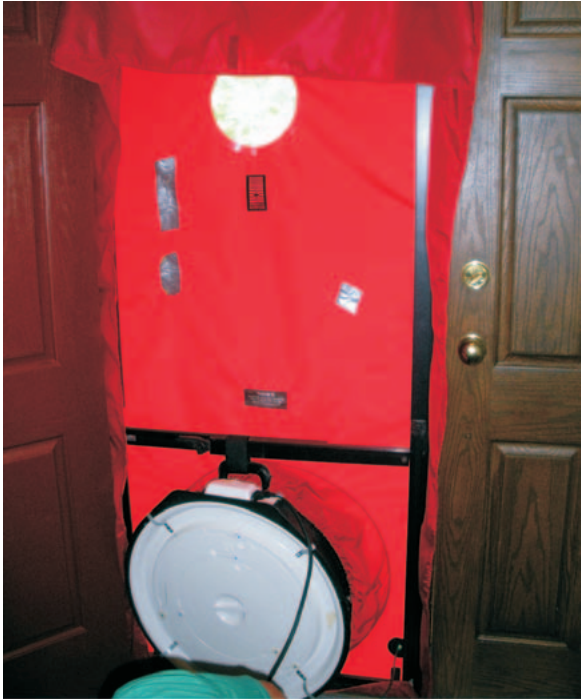
Figure 12: Blower door tests are the most common method to measure air leakage
